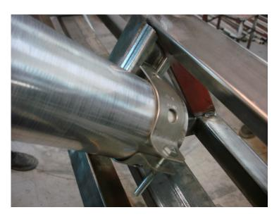
Before placing the trumpets it's important to check that the speakers are placed on their site, at the mouth of the trumpet. The clamps when are placed, also secure the speakers in place.
