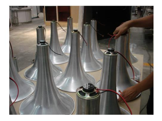
The metal structure has to be assembled before attaching the trumpets with the clamps. In order to facilitate positioning the trumpets it is convenient to set the structure in a horizontal position over sawhorses. Once the trumpets were placed, the next step would be passing the speaker wires through the center of the structure and make the connections following the labels instructions.
